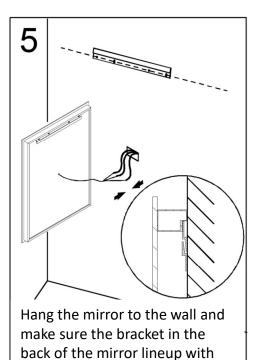
Press the mirror down slightly and make sure the brackets fit properly.
