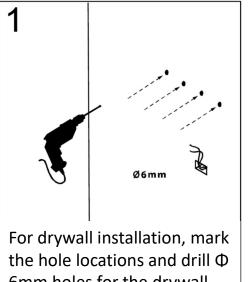
6mm holes for the drywall anchors. Install a junction box behind the mirror for power connections.
